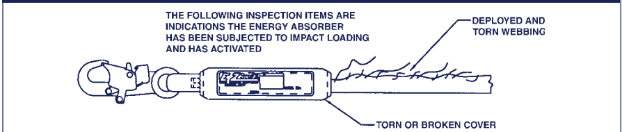
Figure 13 - Inspecting the Energy Absorber for Activation
